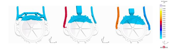
Here these same arrangements are analyzed for air pressure as the mold is filled. The colored alterations in the ingate system indicate gases are escaping against the fluid flow, which should be monitored for non-fill.
