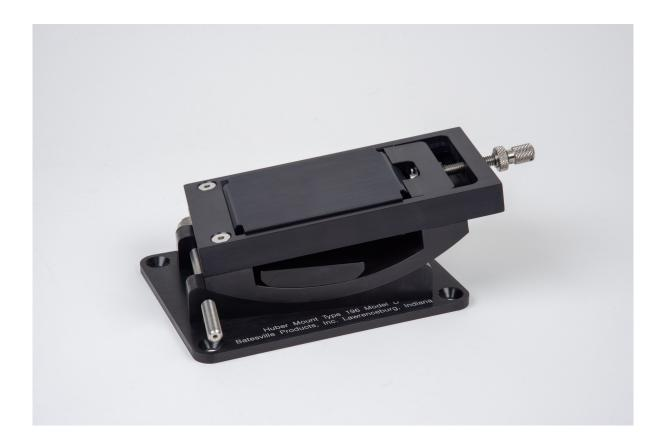
When instruments are too heavy and forces are too great for the 159-P mount, you need to upgrade to 196-D. The Type 195 Model D mount incorporates a worm gear adjustment of the elevation axis, allowing for finer adjustment.
